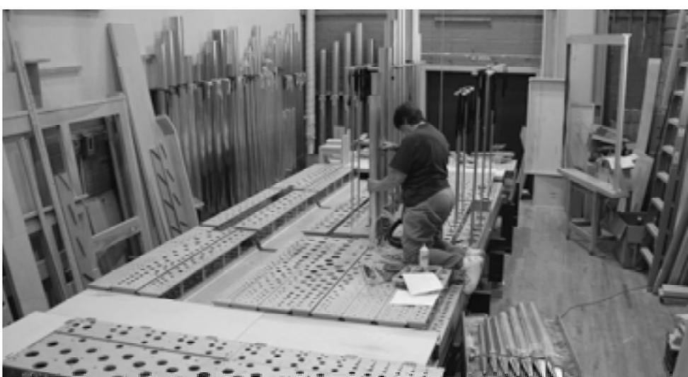
*Racking pipes on the Pedal and Great windchests*
